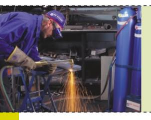
In oxy-acetylene applications, keep safety in mind. Flashbacks occur when the flame passes right through the tip and torch into the hose. It can be very dangerous as it may cause the cylinder to explode. Use flashback arrestors to protect the operator from the hazards of flashbacks.
